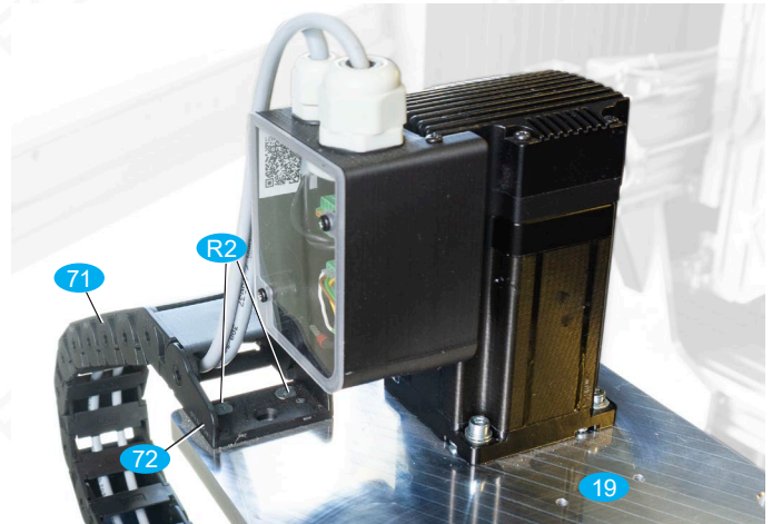
Fig. 6: Mounting drag chain on motor flange
