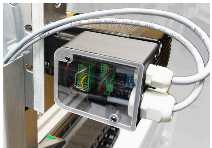
Fig. 11: The cover protects against dust and chips
