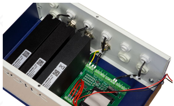
Image 17: Attached power amplifiers
