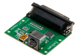
Image 9: Board with adapter module, here for Benezan / Beamicon. In front a module for Estlcam for comparison.
