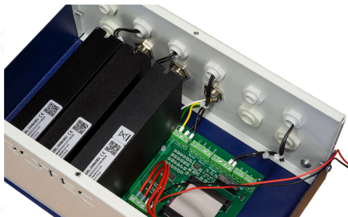
Image 17: Attached power amplifiers
