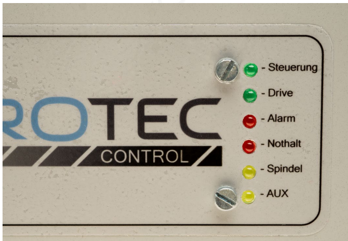
Fig. 31: Status LEDs show the operating status
