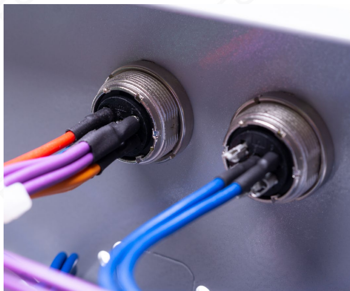
Fig. 16: Each pin individually insulated with shrink tubing
