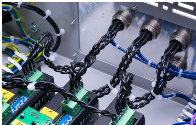
Fig. 18: Power lines are twisted in pairs
