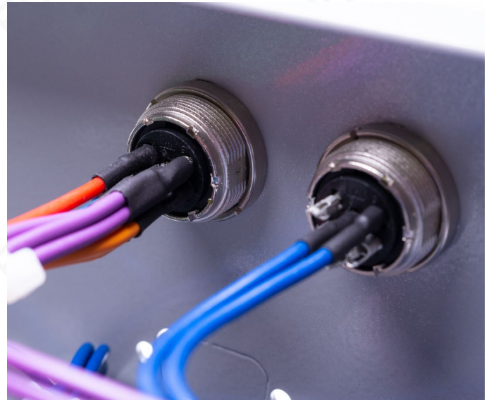
Fig. 19: Each pin individually insulated with shrink tubing
