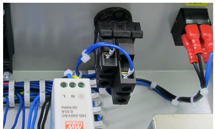
Fig. 4: Assembly of button, LED element, contact element
