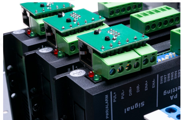
Fig. 9: Mounting the RJ45 adapter on the terminal block
