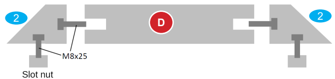
Fig. 4: Pre-assembly of the stiffeners
