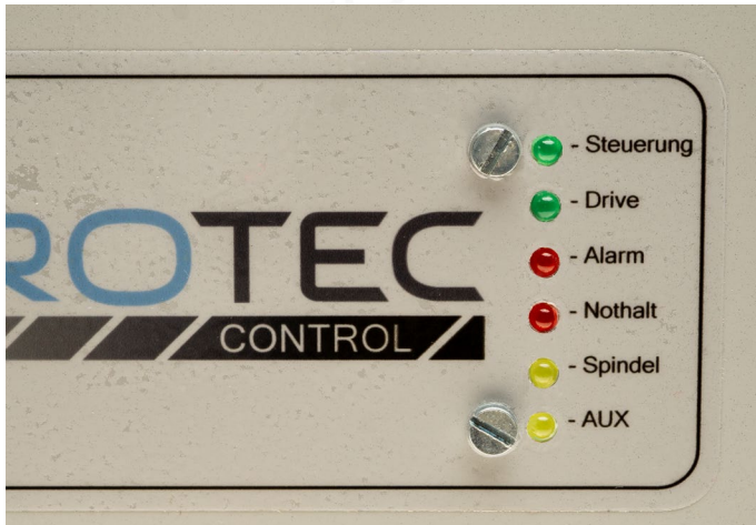
Fig. 31: Status LEDs show the operating status
