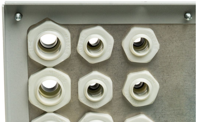
Fig. 15: Orientation of the left nuts to match the opening
