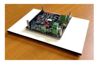
Step 6. Mount the breakout board and fix the board with the four M3 screws
