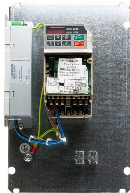
Figure 11: Line filter and frequency converter, mounted and partially wired
