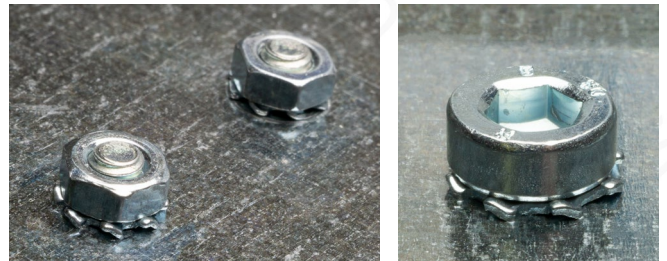
Figure 6 and 7: Shield connection clamps mounted with tooth lock washers, Toothed washer under the head of the earthing screw
