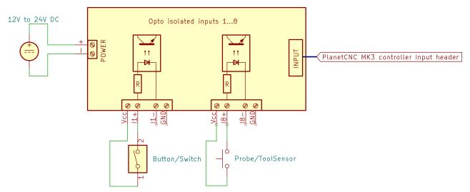
\*Requires "-" jumper on the bottom side to be soldered for both inputs
