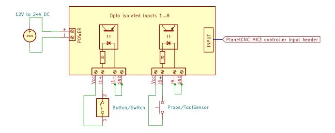
Schematic below describes the use of OptoIso Input adapter with NPN and PNP proximity sensor.
