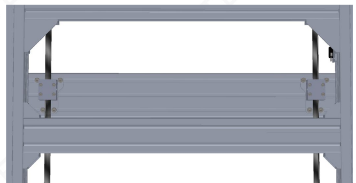
Fig. 4: Connection of portal and recirculating ball nuts
